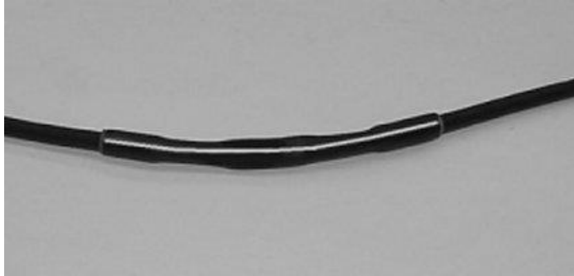
Center Heat Shrink Tube Over Cable
