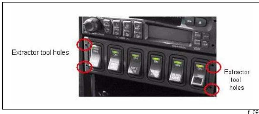
To remove individual switches or blanks from a switch pack, squeeze the locking tabs on the rear of the switch or blank (top and bottom) and push it from the housing.
