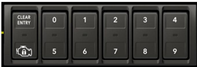
The red ENGINE STOP indicator of the ENGINE STOP/CLEAR ENTRY switch flashes to alert the driver that the theft deterrent code must be entered (within the pre-programmed time delay or the engine will shut down). The momentary CLEAR ENTRY position is pressed whenever the driver needs to clear a failed code so that the correct code can be re-entered.
