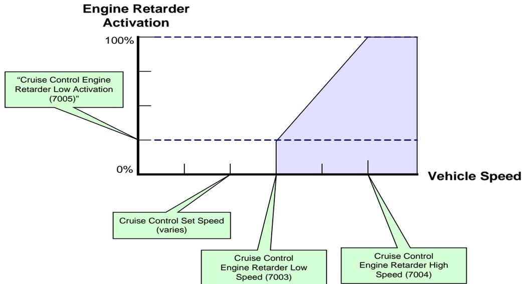
The following programmable parameters, shown in the graph, are customer adjustable. Default settings are used in this example:
